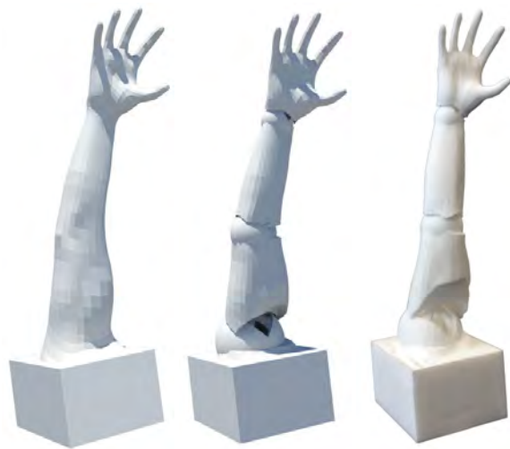
(a) Arm model (input, articulated, 3D print)
