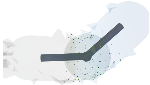
Figure 9: The result of our sphere fitting on a simple mesh; green points indicate intersection points.
