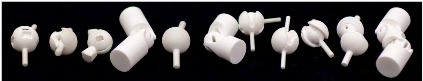
Figure 2: A range of test joints fabricated to informally explore physical properties of various joint designs.
