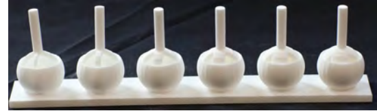
(b) Band thickness calibration set
