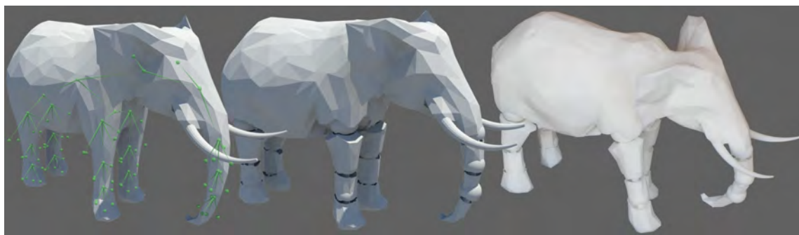
Figure 1: Starting from a 3D mesh (left), our system allows to intuitively add 3D-printable joints (center) that, when 3D-printed, create a functional, posable model with joints that exhibit internal friction. The model leaves the printer ready to use; no manual assembly is required.
