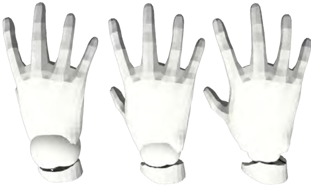
Figure 10: Three differently scaled wrist joints, at 120%, 100%, and 80% of the sphere fit radius.
