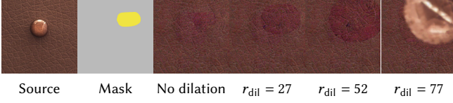
Fig. 23. Failure case for Diffusion Texture Painting [Hu et al. 2024]. The results are generated with a progressively dilated mask. Only at the largest size (dilated by 77 pixels), the feature is actually painted.
