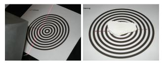
Figure 4: To reduce scanning time, a target records scanner settings for several laser positions (left). The operator uses this target to set the laser range for each fragment, so that only the relevant portion of the viewing volume is scanned (right).
