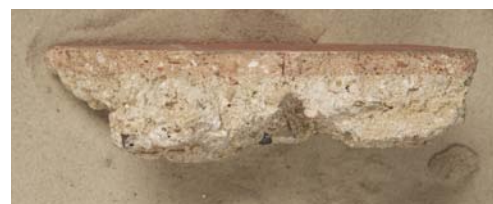
Figure 2: Side view showing the two layers of mortar that identify this painting ( Copyright Gallo-Romeins Museum Tongeren ).
