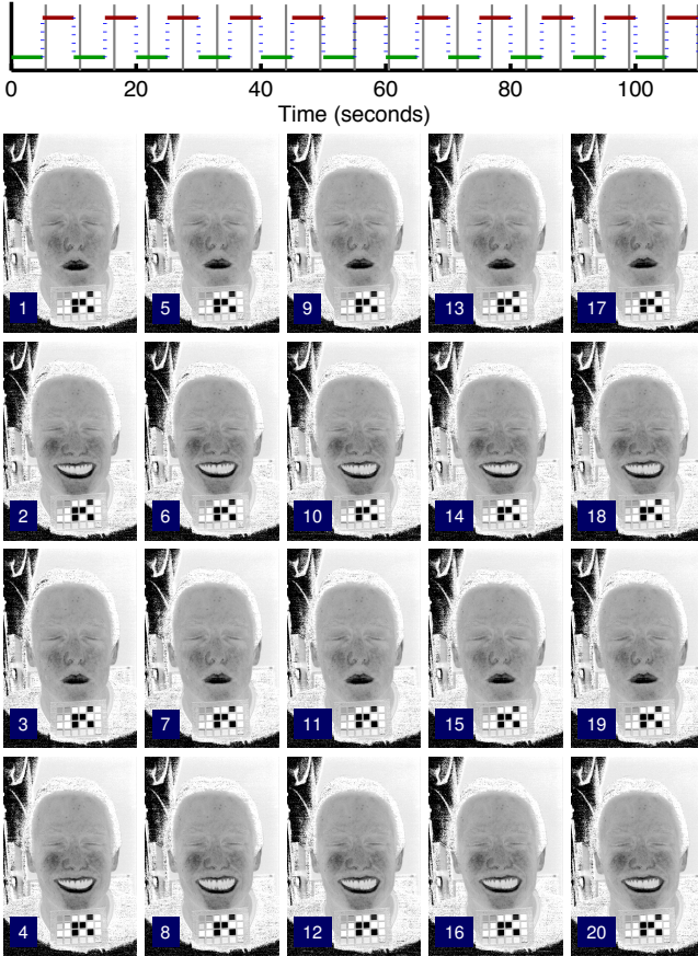
Figure 6: Our time multiplexing scheme. Top: We sample the expressions at varying time offsets from the expression transition. Bottom: The images were taken in column-major order (as numbered), with a short phase shift between acquisition and expression changes. This gives a consistent 5-image temporal sequence of four expressions (neutral/smile/neutral/smile) when arranged in row-major order.
