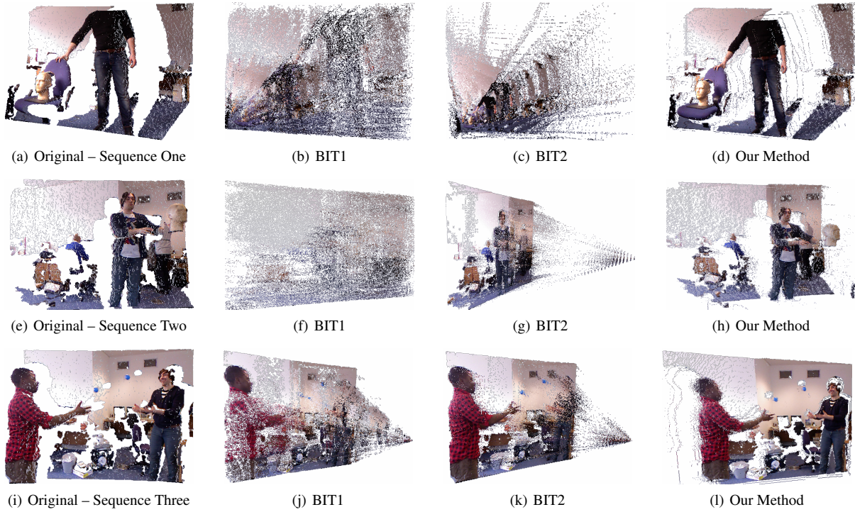
Figure 11: Comparison of reconstructed depth maps using different depth coding strategies and JPEG compression (75%).
