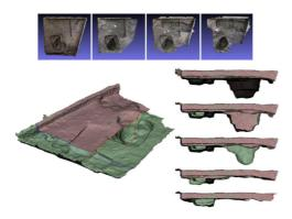
**Figure 25:** Monitoring the excavation with photogrammetric approaches. Top: acquired 3D model of the same archaeological site in different times, showing the evolution of the excavation. Bottom: interactive slicing visualization to highlight the evolution of the excavation in specific areas of the site. Courtesy of Dellepiane et al. Reproduced from [DDUC\*13], Copyright © 2013, published by Elsevier Masson SAS. All rights reserved.
