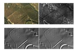
**Figure 26:** Analysis of airborne laser scanning data for archeological sites identification. Top: aerial and intensity image of the studied area. Bottom: resulting DTM after processing, which shows possible archaeological sites once the information of forested areas has been removed. Courtesy of Doneus et al. [DB06] (Copyright Eurographics Association).
