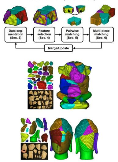
**Figure 7:** Reassembling fractured objects. Top row: high level overview of the reassembly pipeline. Middle and bottom row: two examples of reassembled objects. For each object the image shows the photo (bottom left) and the 3D models (top left) of the fragments, and the final assembly (right). Courtesy of Pottmann et al. [HFG\*06] © 2006 Association for Computing Machinery, Inc. Reprinted by permission.
