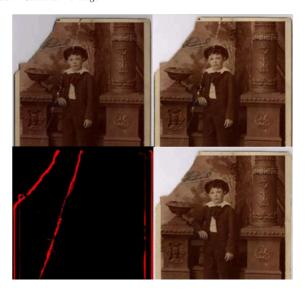
**Figure 14:** Document restoration. First row: two images acquired with a flatbed scanner that incorporates two separate and independently controlled illumination bulbs. By using photometric stereo [Woo79] tears and creases are extracted (low-left), and infilling algorithms are applied to digitally restore the image (low-right) [PMW\*09] (With kind permission from Springer Science and Business Media).
