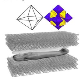
**Figure 24:** Geometric analysis for packaging applications. Top: the octahedron, which is the basic unit that has been used to build the 3D printed package. Bottom: The final structure ready to print. Courtesy of Sá et al. [SEG\*12] (Copyright Eurographics Association).
