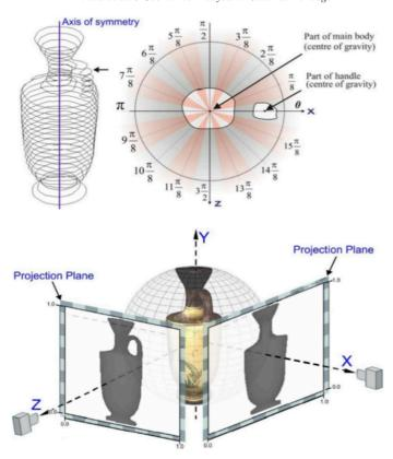
**Figure 15:** Pottery shape descriptors. Top: set of curves by intersecting the pottery and a plane orthogonal to its axis of symmetry. Bottom: set of two depth maps by projecting the object onto two orthogonal planes. Courtesy of Koutsoudis et al., © [2010] IEEE. Reprinted, with permission, from [KPC10].
